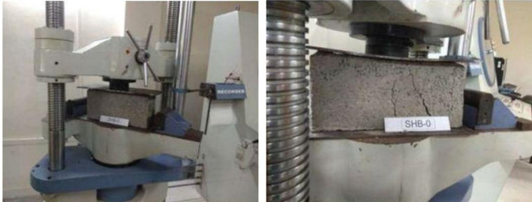
**Figure 2: Testing of slag hollow blocks**
