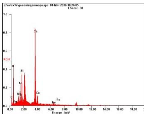
**Figure 5: Energy Dispersive X-Ray Analysis image of slag concrete**
