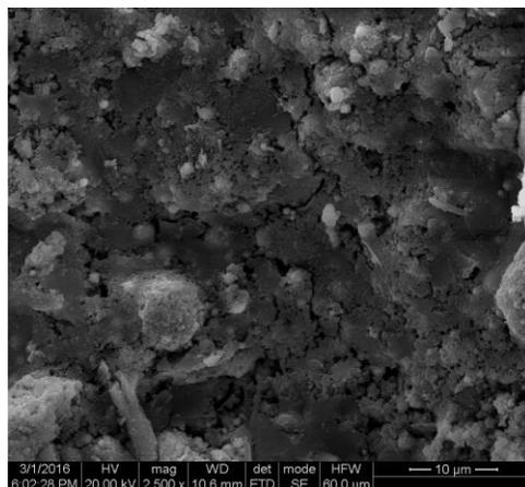
**Figure 4: Scanning Electron Microscope image of slag concrete**
