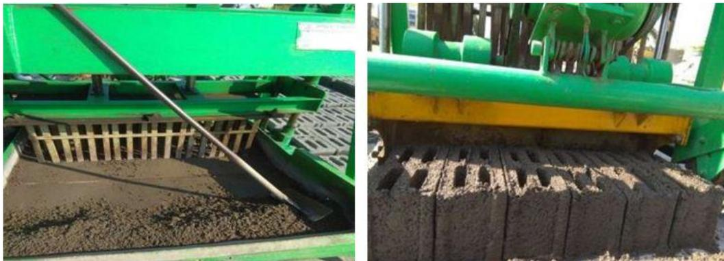
**Figure 1: Preparation of slag concrete hollow blocks**
