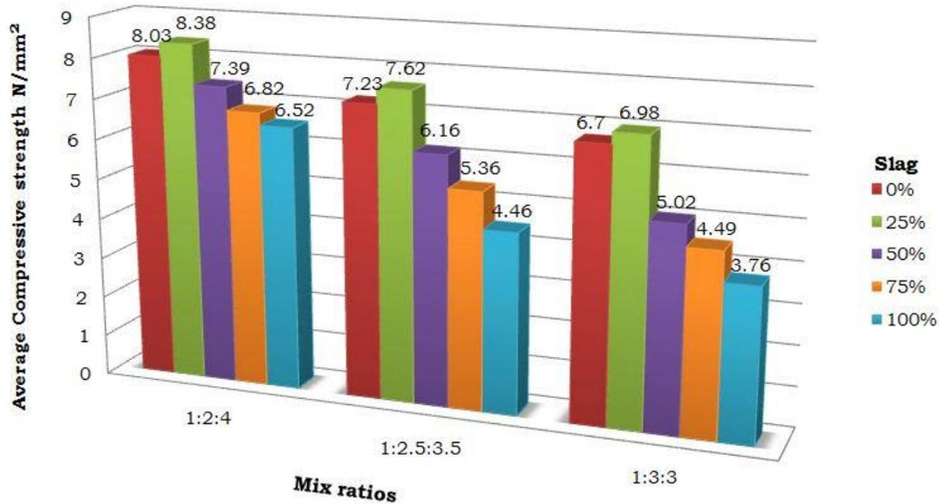
Figure 3: Compressive strength of slag hollow blocks
